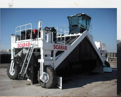
Central Valley Wastewater Facility in Salt Lake City uses a covered aerated static windrow design, and is using a windrow turner so that they don't have to move the windrows with a loader
