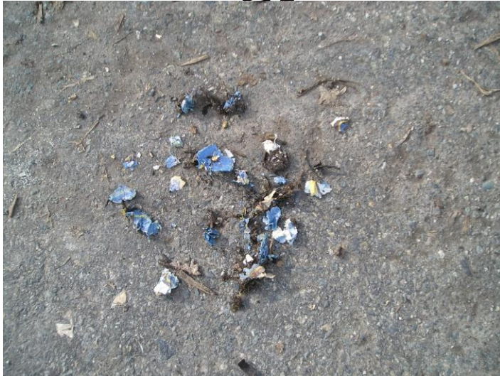
Frito Lay compostable bag fragments after 45 days
