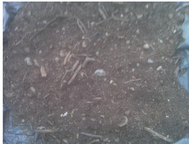
10.5 oz Frito Lay Compostable Bag 69 days: Completely mineralized and no fragments remaining
