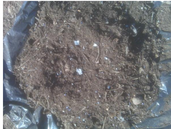
1 oz Frito Lay Compostable Bag 35 days: Completely mineralized and no fragments remaining
