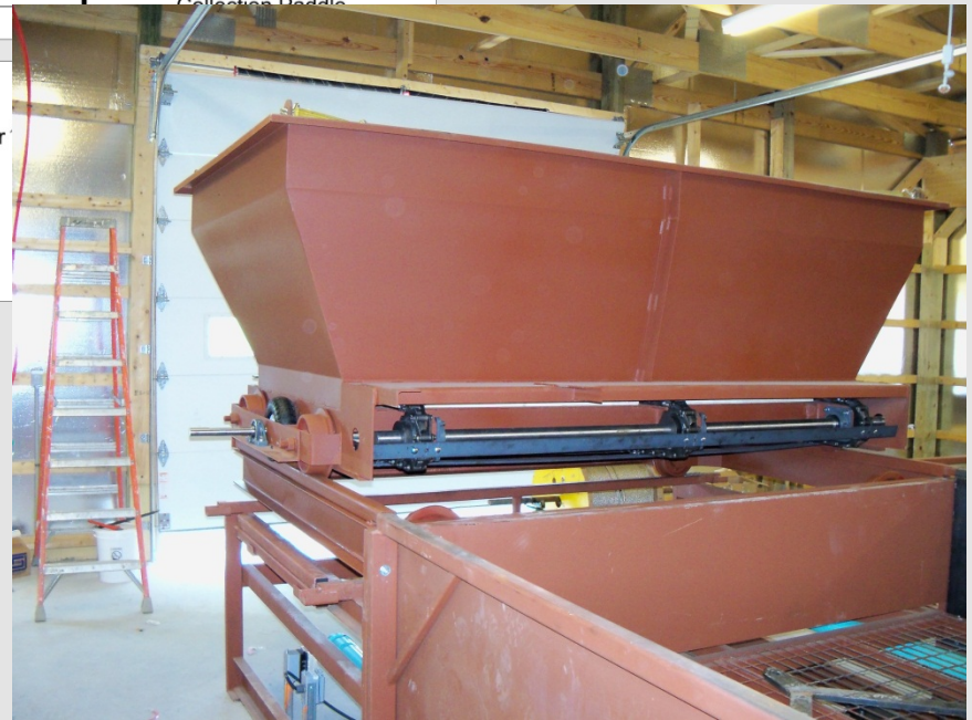
6" Concrete Floor Continuous-Process, Flow-Through Earthworm Vermicomposting Digester
