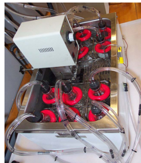
Water condenser and ammonia trap (9° C.)
