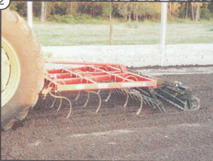
Raking & mixing wet material with dry accelerates the drying process (even on rainy days)
