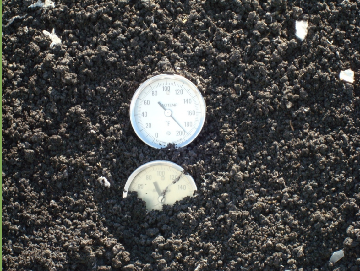
Temperatures in the aerated static pile.
